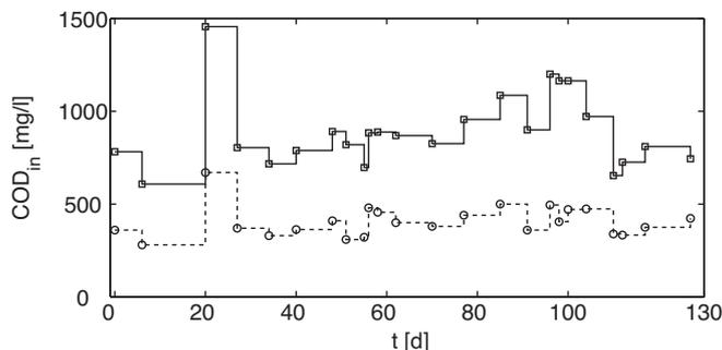
**Fig. 1.** Unsteady COD inflow concentrations. The squares and circles represent the measured data from Galvão and Matos (2012) for group A and B, respectively. The continuous and dashed lines figure the inflow trend assumed in simulations for A and B, respectively.
